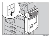
Open the machine's right cover by pushing up the catch.
